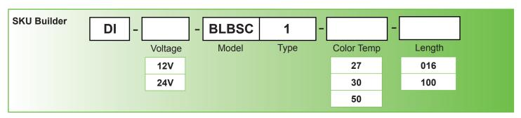
Example: DI-12V-BLBSC1-27-16 = Diode LED, 12 Volt, BLAZE™ BASICS, Type 1, 2,700° CCT, 16.4 foot spool.
